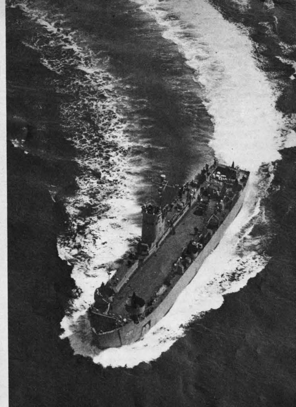
Halfway step between an LST and an LCT, the new LSM combines the best features of each. She is an ocean-going vessel with a long range and adequate carrying capacity but has greater speed than the lumbering older LST.
